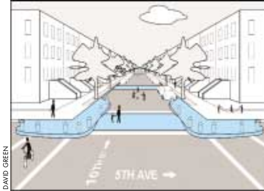
A traffic calming scheme prepared for a NSN member. This design uses neckdowns, a raised crosswalk, and speed humps to create a "slow street" where neighborhood residents, not speeding cars, come first. The NSN is pushing for this kind of streetscape all over the city.
