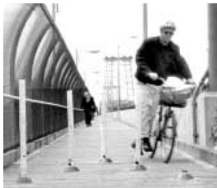
Flexible bollards, like these on the Williamsburg, slow cyclists and eliminate the need for “dismount” signs.
