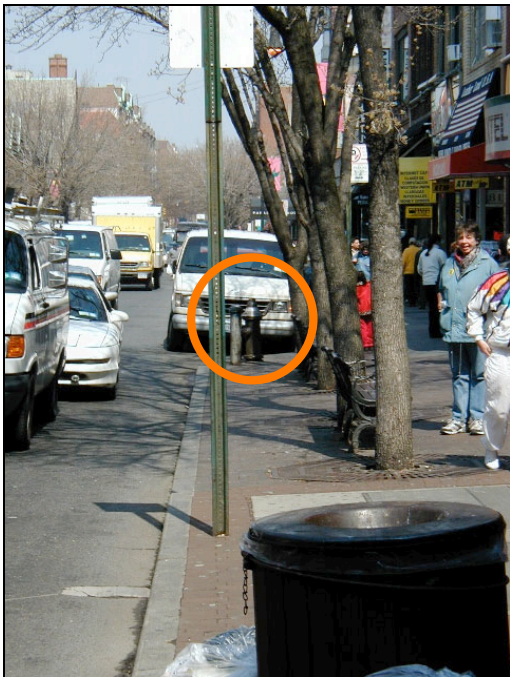
Figure 5: Hydrant on Curb Extension, 82nd Street
